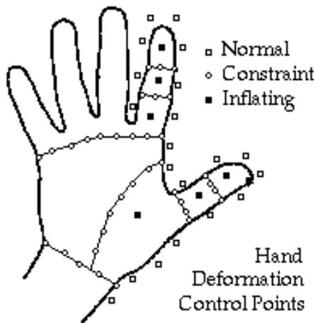
**Figure 3.** The 3 types of control points
